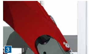
3 Reinforced arm on connection to clamp body
